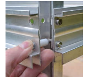
Nylon spacer on bolt
