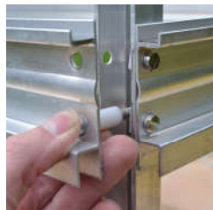
Nylon spacer on bolt
