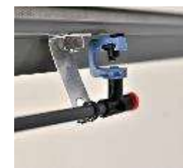
Nozzle strapped to 'L' bracket—position x
