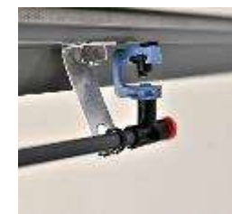
Nozzle strapped to 'L' bracket—position x
