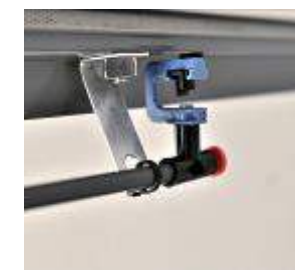
Nozzle strapped to 'L' bracket
