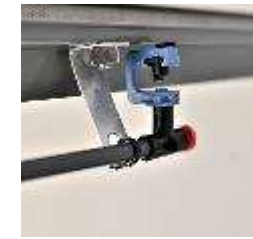
Nozzle strapped to 'L' bracket—position x
