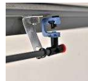
Nozzle strapped to 'L' bracket
