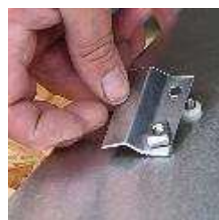
Nylon spacers on infill plate
