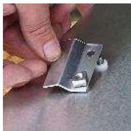
Nylon spacers on infill plate
