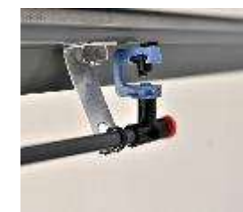
Nozzle strapped to 'L' bracket—position x
